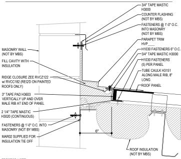
ERECTOR NOTE: INSULATION TIE-OFF SHOWN IS ONE METHOD. MAY REQUIRE DIFFERENT METHOD BASED ON SEQUENCE.H1020 FASTENERS (PURLINS) & H1070 FASTENERS (JOISTS) WITH H2200 INSULATION WASHERS HAVE BEEN SUPPLIED 12" O.C. FOR INSULATION ATTACHMENT
