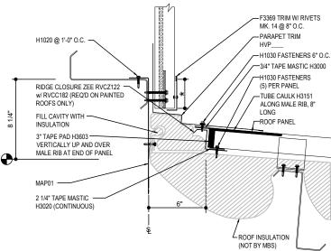
ERECTOR NOTE: INSULATION TIE-OFF SHOWN IS ONE METHOD. MAY REQUIRE DIFFERENT METHOD BASED ON SEQUENCE.H1020 FASTENERS (PURLINS) & H1070 FASTENERS (JOISTS) WITH H2200 INSULATION WASHERS HAVE BEEN SUPPLIED 12" O.C. FOR INSULATION ATTACHMENT
